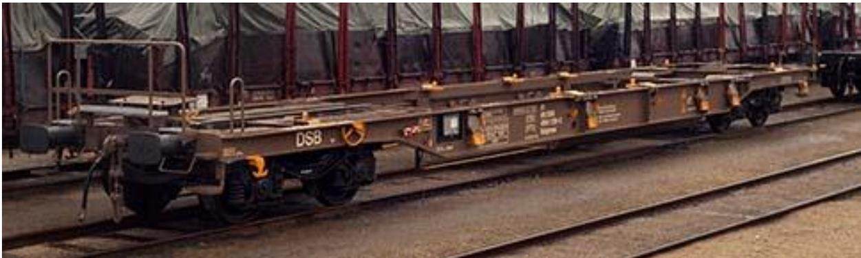
The cargo wagon, specifically, is properly used for the transport of cargo units (containers and swap bodies), together with goods and vehicles in other non-intermodal containers. It has not mobile parts and the loading is possible only vertically.
